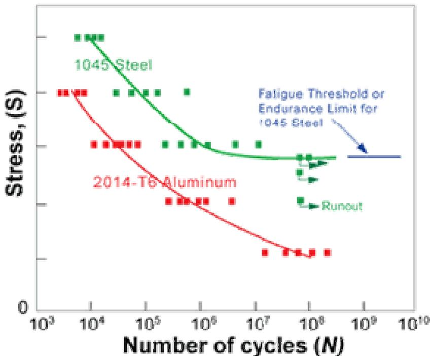
**Figure 3: Aluminium Fatigue Endurance**
