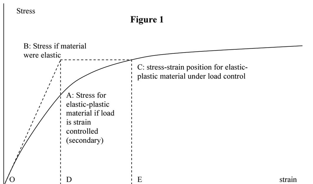
Recall from the homework of session 15 that, as a rough rule-of-thumb, the elastic-plastic J is proportional to the area under the load-displacement curve – which might be roughly proportional to the area under the above stress-strain curve. So we would expect the relative magnitudes of the J's for (a)elastic-plastic strain control, (b)elastic material, and, (c)elastic-plastic load control, to be in the order of the corresponding areas,
