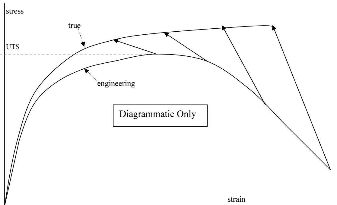
True stress – true strain curves tend to be monotonic (i.e. never decreasing) in contrast with the maximum at the UTS displayed by the engineering stress-strain curve.
