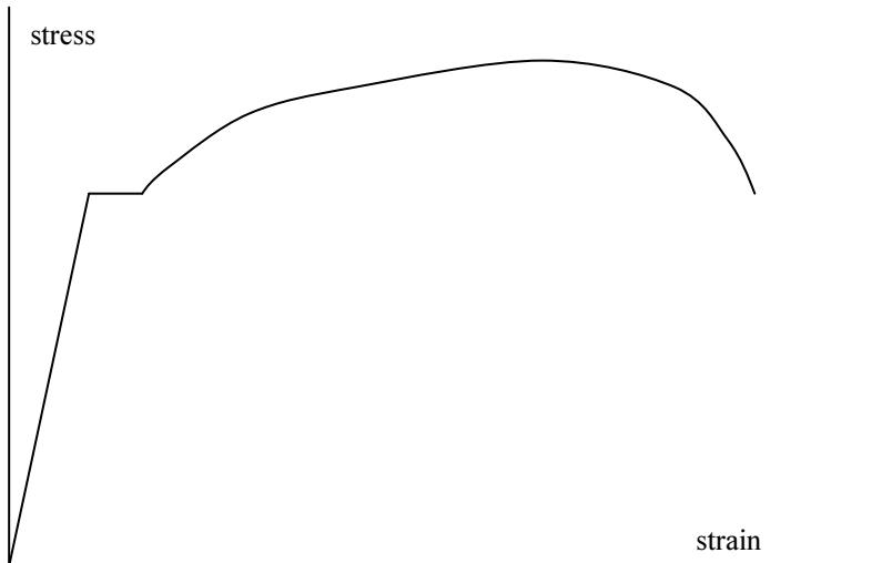
In this case it is clear how the yield stress is defined. Other steels, typically austenitics, do not have a distinct yield point but merely display a stress-strain curve of increasing curvature,
