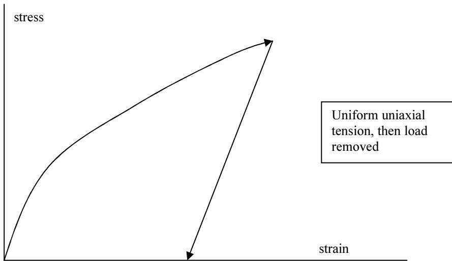
But note that we end up with zero stress only because the uniaxial specimen was assumed to be uniformly stressed. So, a return to zero load means a return to zero stress.
