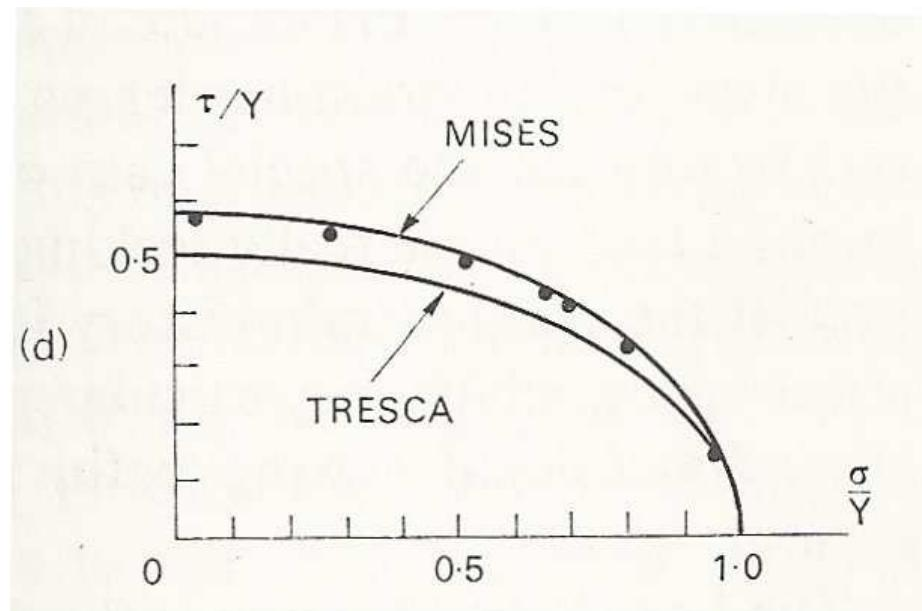
These tests considered cases of combined tension & shear - achieved using a tension-torsion machine. Note that such tests produce a *smaller* ratio of hydrostatic to Mises stress than simple tension (negative constraint). In such cases it was found that the Tresca criterion generally underestimates the load at yield whereas the Mises criterion is quite good.
