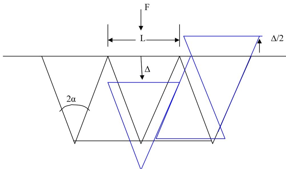
The blue lines show the displaced triangles – on one side only – due to a downwards displacement of the indenter by  $\Delta$ . (*Apologies for the distortions – my skill with WordArt is poor*).
