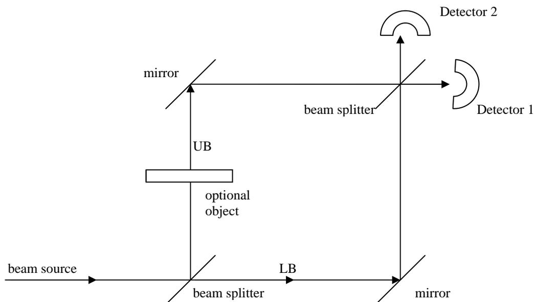
If the final beam splitter were omitted, detector 1 would measure only photons taking the path UB, and detector 2 would measure only photons taking path LB. Both would occur with equal frequency (assuming the first beam splitter is 50/50). There is no interference (rather trivially in this case since, in the absence of the final beam splitter, the two paths are never brought together in order to interfere).
